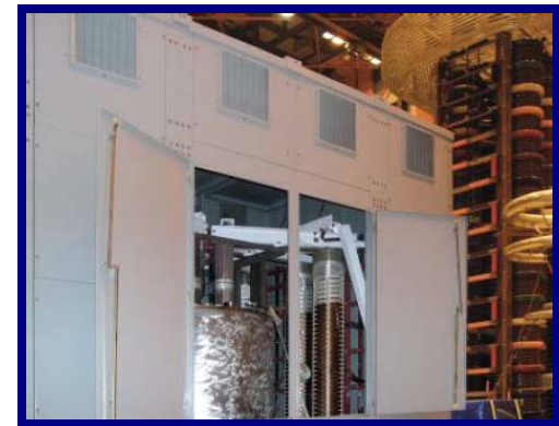
Zenergy's FCL Testing at PowerTech
